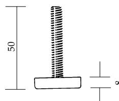
Screw socket for adjustable foot for hexagonal profile
