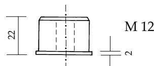
Screw socket for adjustable foot for octagonal profile
