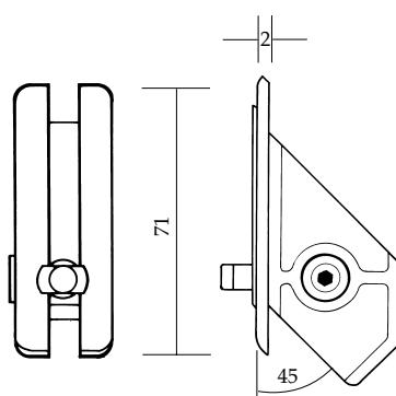
Lock for curved beam profiles, unassembled
