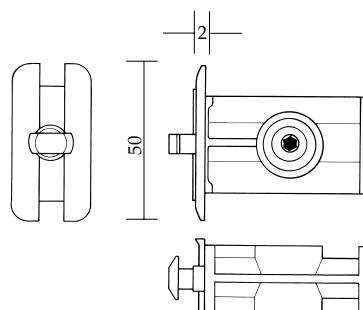
Lock 45 for 50 mm beam profiles, unassembled
